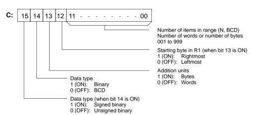
**Number of Items in Range** The number of items within the range (N) is contained in the 3 rightmost digits of C, which must be BCD between 001 and 999. This number will indicate the number of words or the number of bytes depending the items being summed.
